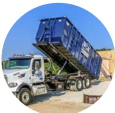
CNG-fuelled WCA waste collection truck with hydraulic tipper engaged
